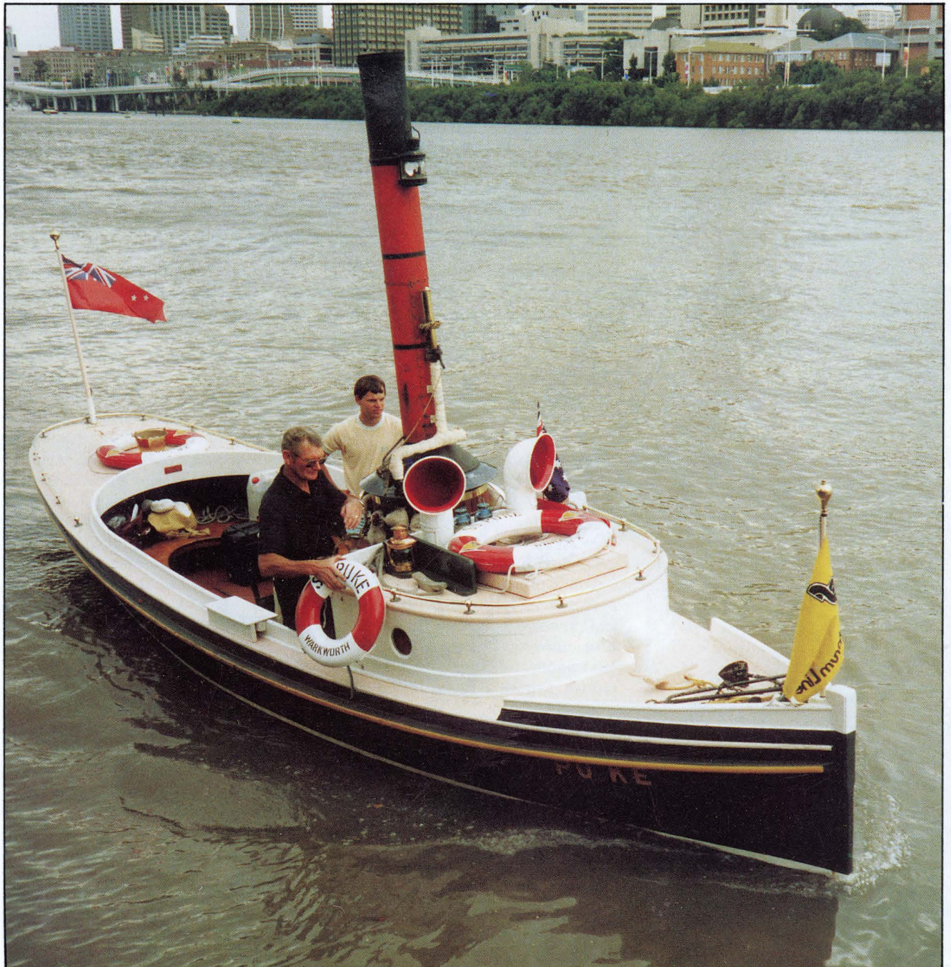
Below & opposite: The PUKE on the Brisbane River during (Expo 88'. She shows the characteristics steam launch features of her time: plumb stem, low free board, long counter, round-fronted cabin and vertical boiler.
